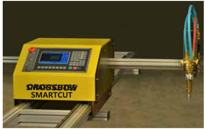
Maximum Oxy-fuel Cutting Thickness of up to 100 mm (4 in.)
