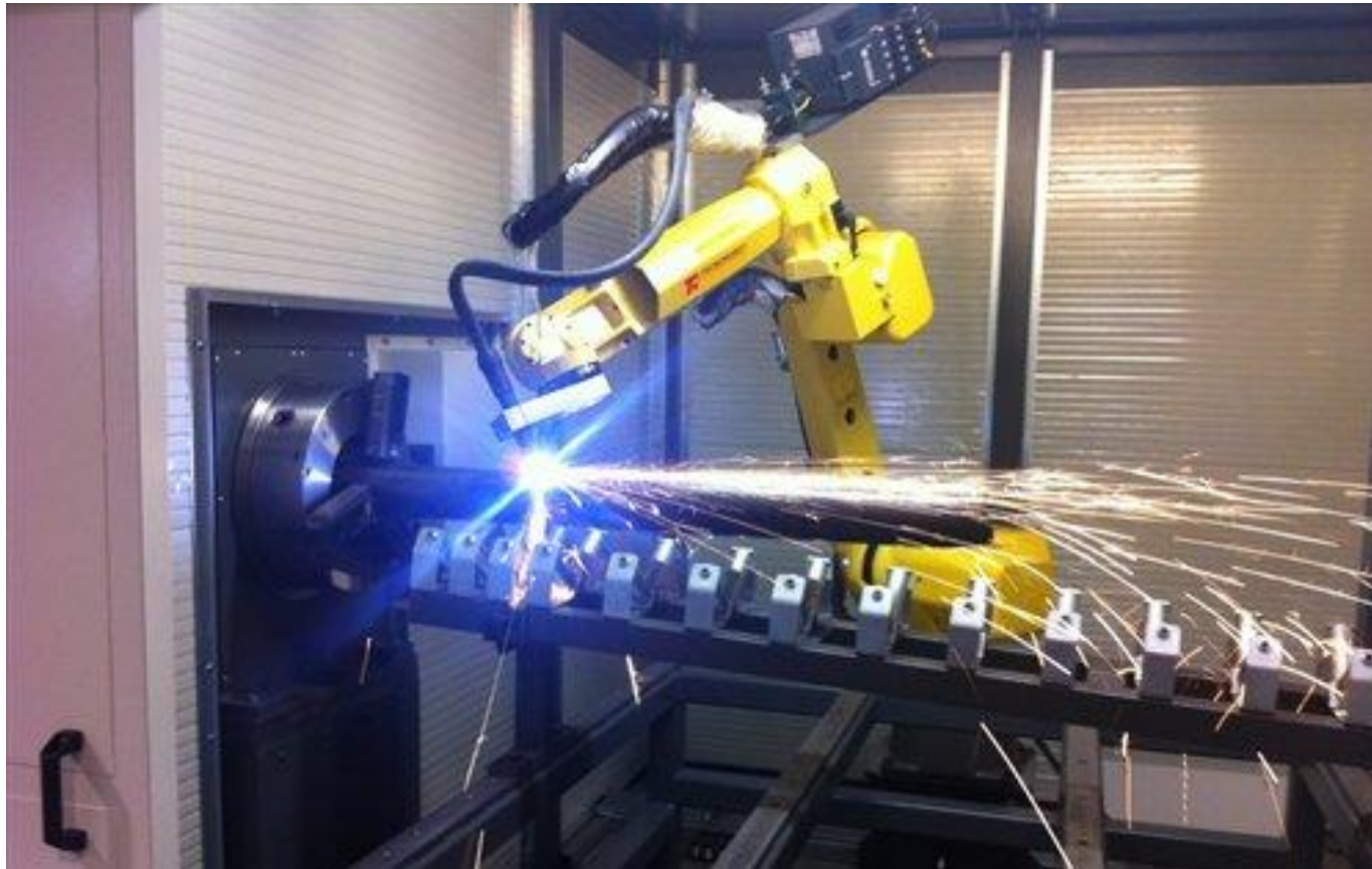
Custom designed robotic tube trimming cell
