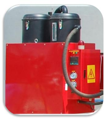
\*Note: For your application, this unit will act as standlone FRU unit which collects the flux through Vacuum from the tray and for feeding the flux is installed with valve, where the customer can collect the flux and load into hopper manually.
