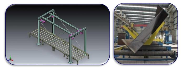
Beam Flippers unit is assembled to the outfeed conveyor of Pull through welder which is used to flip the welded beam to other side for second side welding.
